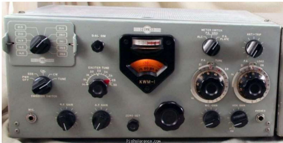
KWM-1 (1957) SSB/CW 20, 15, 10 meters New price $770 About 1150 units produced
