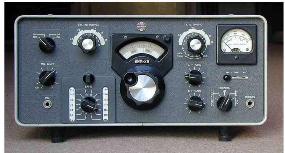
KWM-2 (1959) KWM-2A (1961) SSB/CW 80 - 10 meters New price $1150 2A - $1250 About 26,000 units produced
